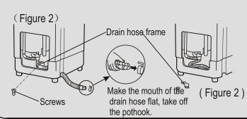
back cover on the cabinet firstly, then push the left the right tab and the upside into the cabinet. Do not do it strongly, and fasten the screws.
